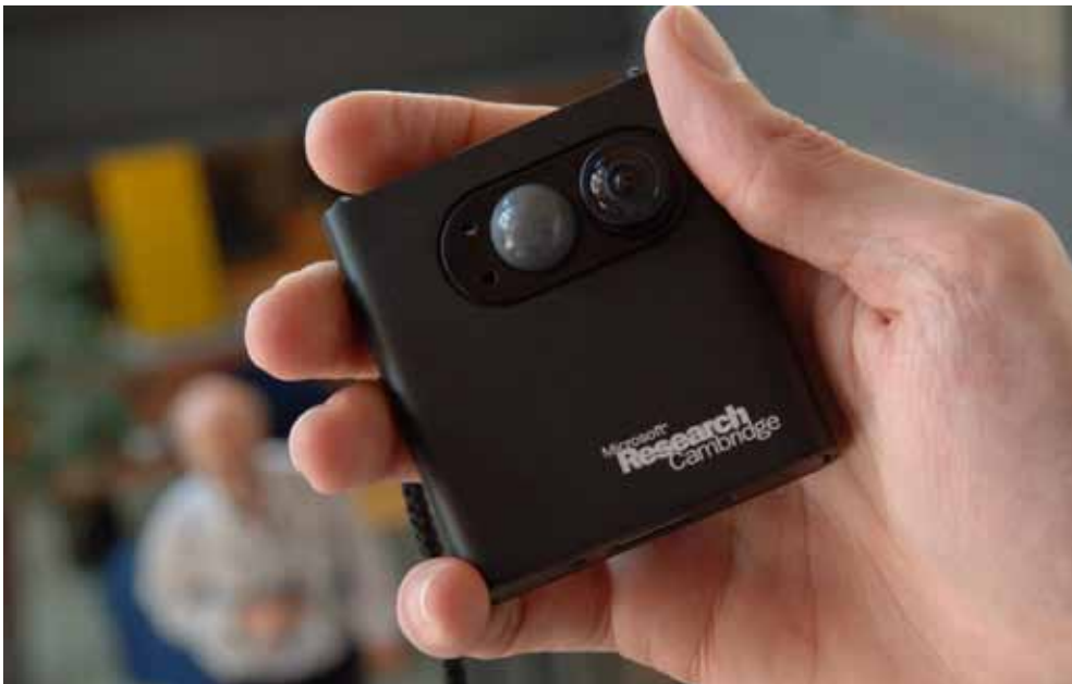
Figure 2.5: Microsoft's Sence Cam, that picks crucial images, and reviews them periodically to awaken and strengthen the memory of the event.
