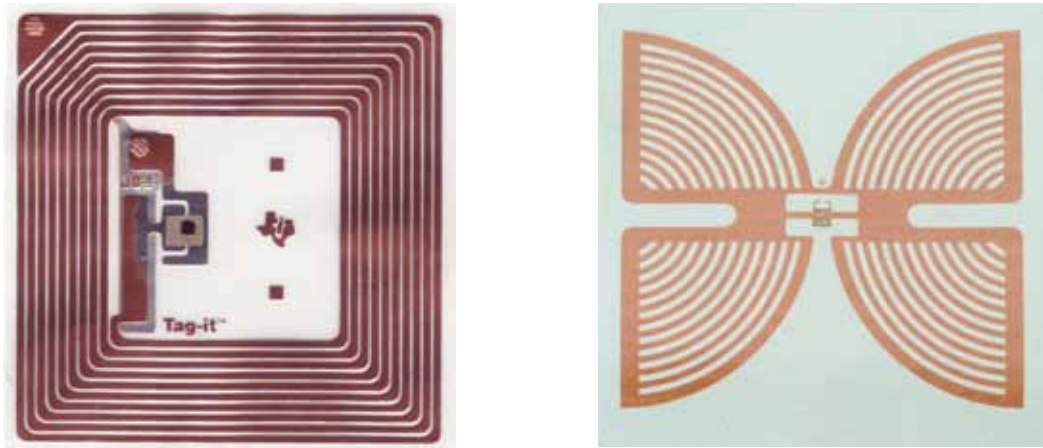
Figure 2.7: Standard RFID Tag. The Antenna is normally moulded as a coil-shaped circuit. With designer's ingenuity, an RFID antenna can be designed in aesthetically way.
